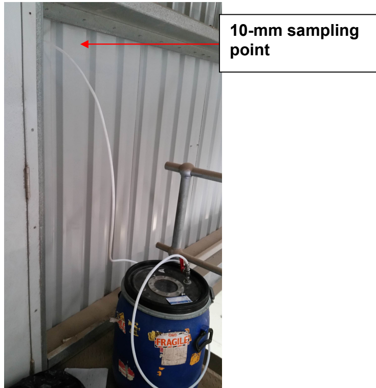
Photo 1 – An example of the roof discharge stack odour sampling point at the BTT Facility
