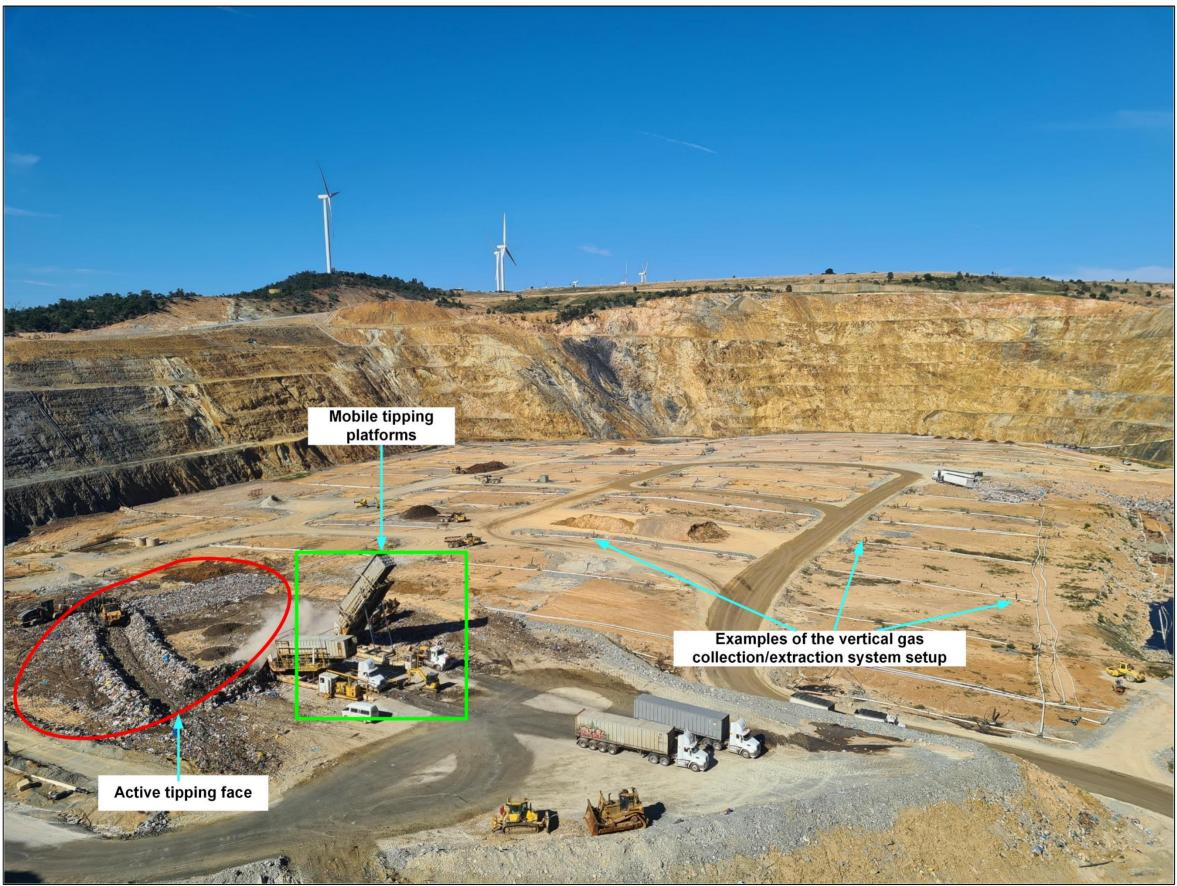
Figure 2.2 – Void layout and operations: 22 March 2022
