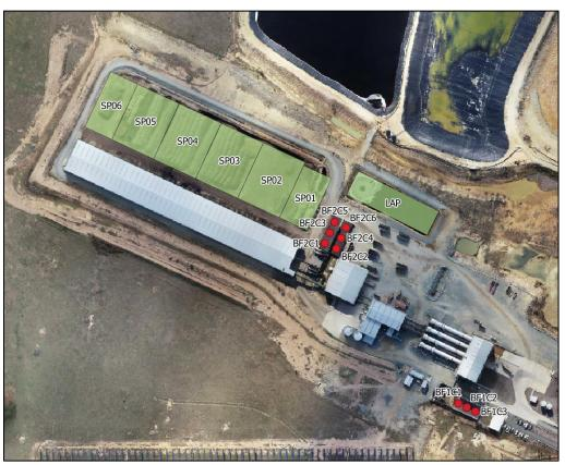
Figure 8.2 - Layout of modelled MBT sources in the Audit
