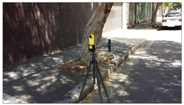
**Photo 7.1 -** Illustrated setup of the Kestrel Anemometer apparatus in operation (**Source**: TOU)
