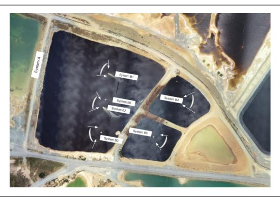
Figure 2.3 – The mechanical evaporation system layout for ED3N (Source: WIP 2020)
