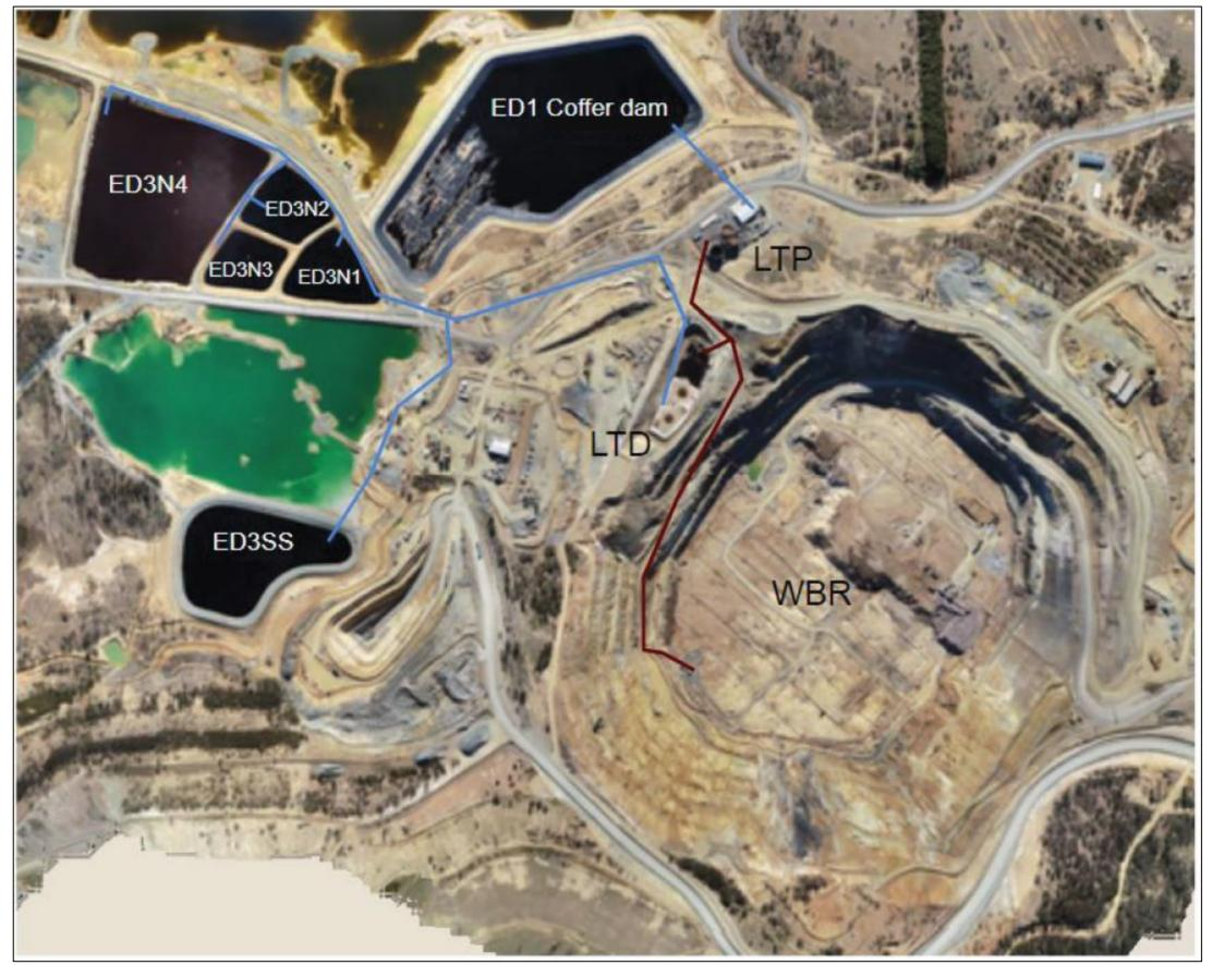
Figure 2.10 - Concept layout of the LMS for the Bioreactor at the Woodlawn Facility (Source: WIP 2020)
