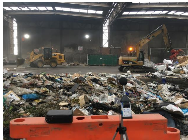
Photograph 3.2: Excavator with grab arm and front-end loader
