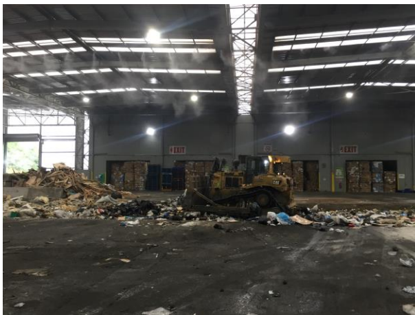
Photograph 3.1: Bulldozer compacting waste
