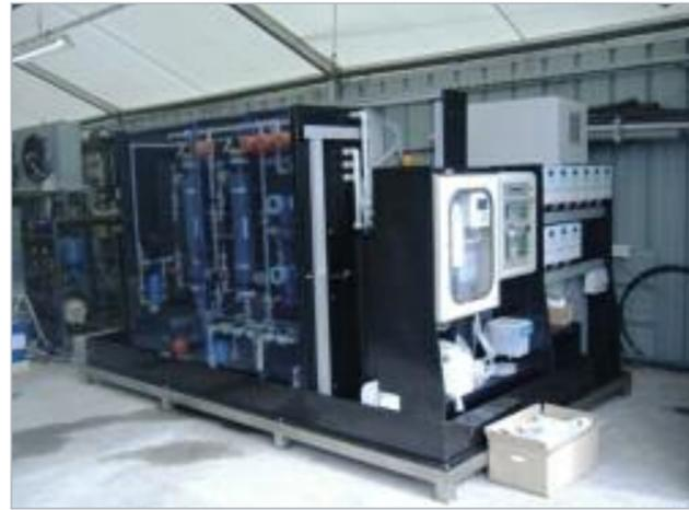
■ Membrane contactor pilot unit
