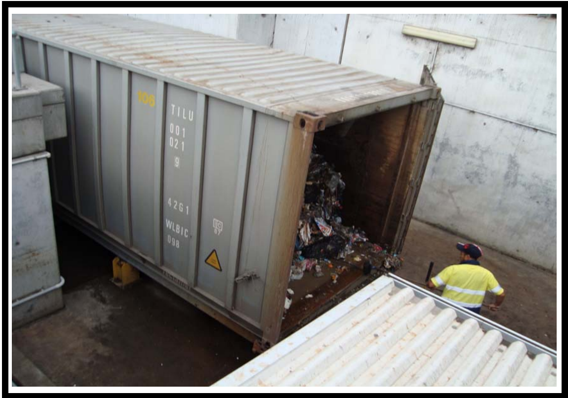
Photo 5: Container with compacted waste 'slug' being tidied prior to transfer to rail car.
