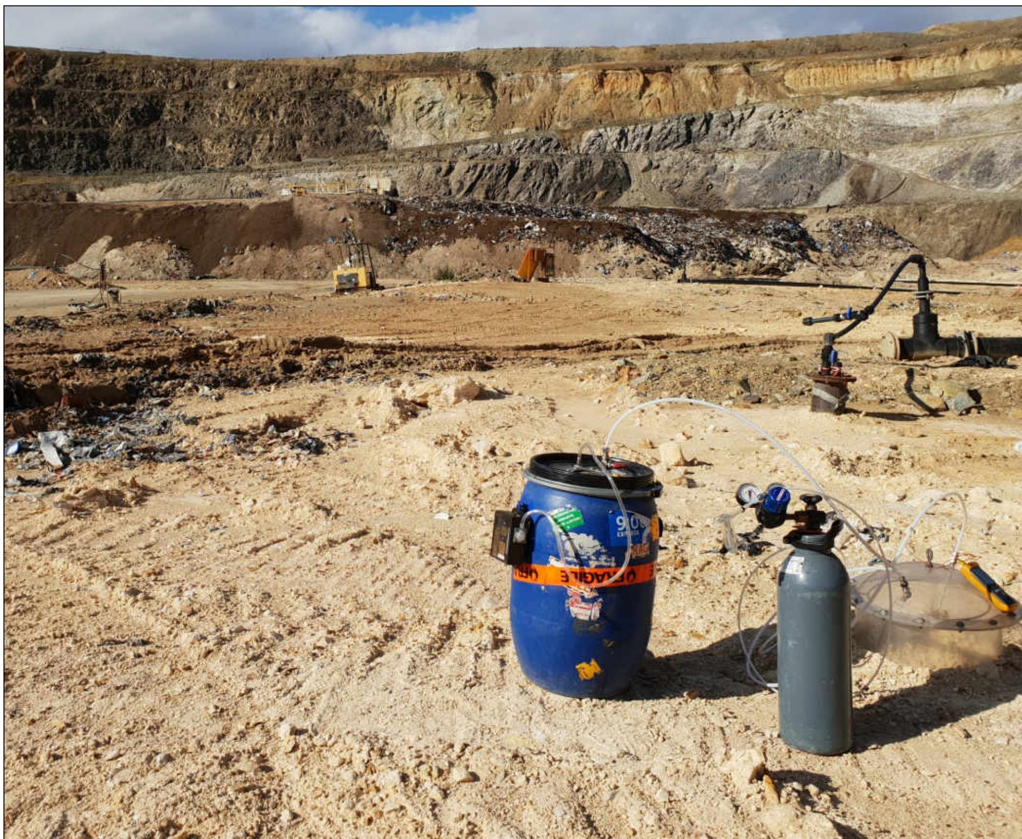
Photo 4.1 – An example of IFH sampling on a solid surface in the Void as occurred on 21 February 2019
