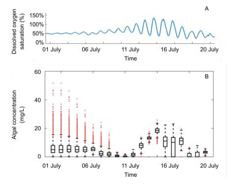
Results of the mathematical model implemented to convert oxygen fluctuations measured by the SWARM buoy (top) into an algal concentration (bottom).
