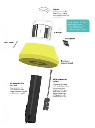
The SWARM buoy was designed to ensure that most maintenance operations can be done from a boat or river/reservoir banks, in particular:
