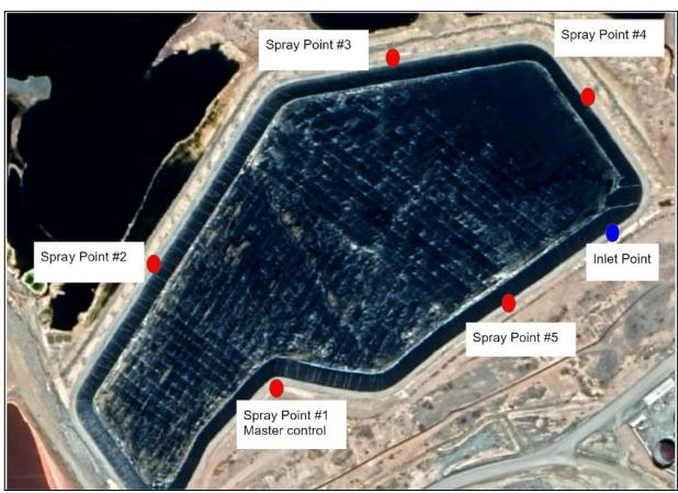
Figure 2.6 – ED1 Coffer Dam: Proposed Evaporation Spray System (Source: WIP 2020)
