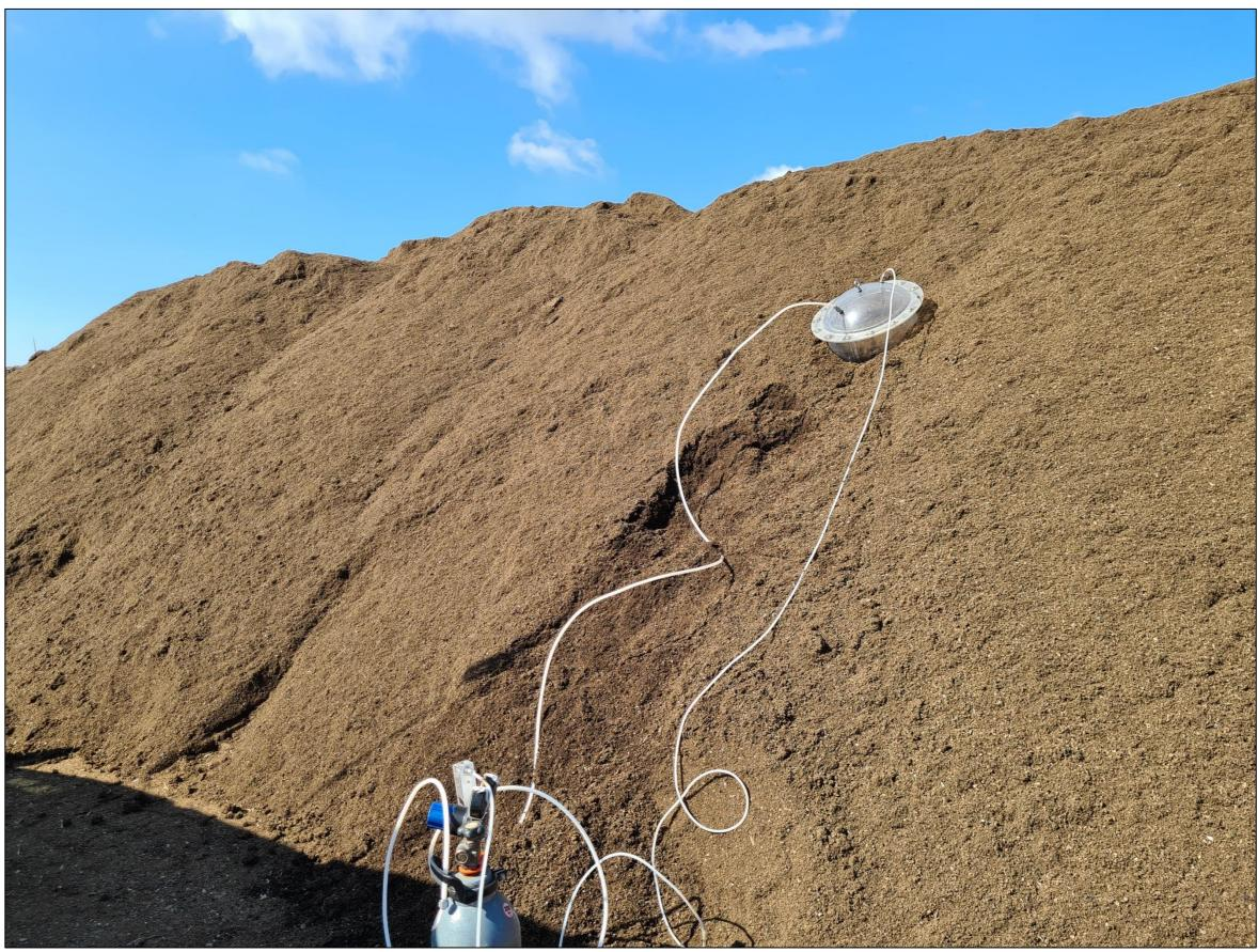
Photo 4.1 - An example of IFH sampling on a solid surface at the MBT Facility as occurred on 11 March 2021
