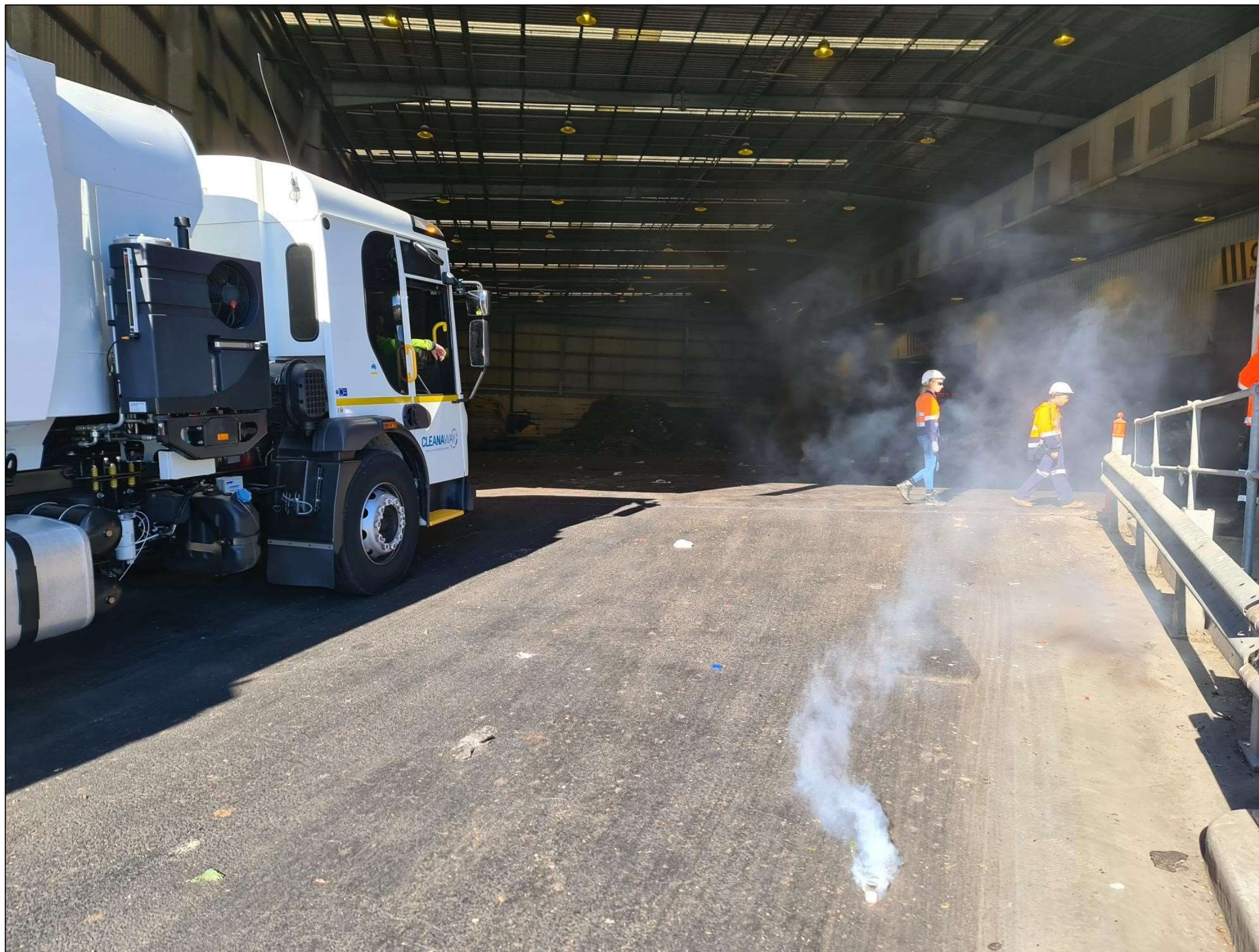
Photo 2 – Smoke testing at the truck entry point of the BTT Facility building enclosure on 14 May 2021
