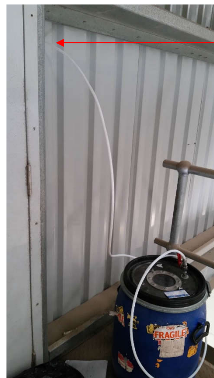
Photo 1 – An example of the roof discharge stack odour sampling point at the BTT Facility
