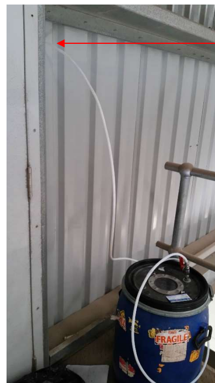
Photo 1 – An example of the roof discharge stack odour sampling point at the BTT Facility
