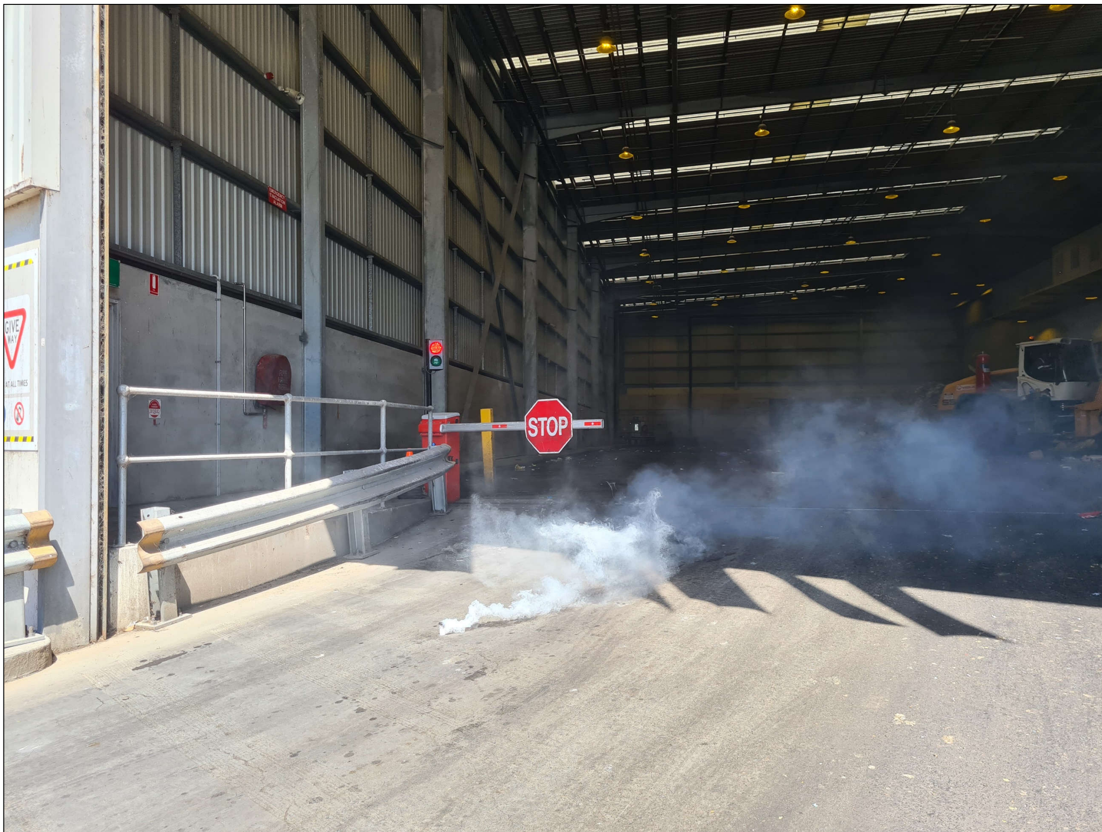
Photo 2 – Smoke testing at the truck entry point of the BTT Facility building enclosure on 1 October 2020
