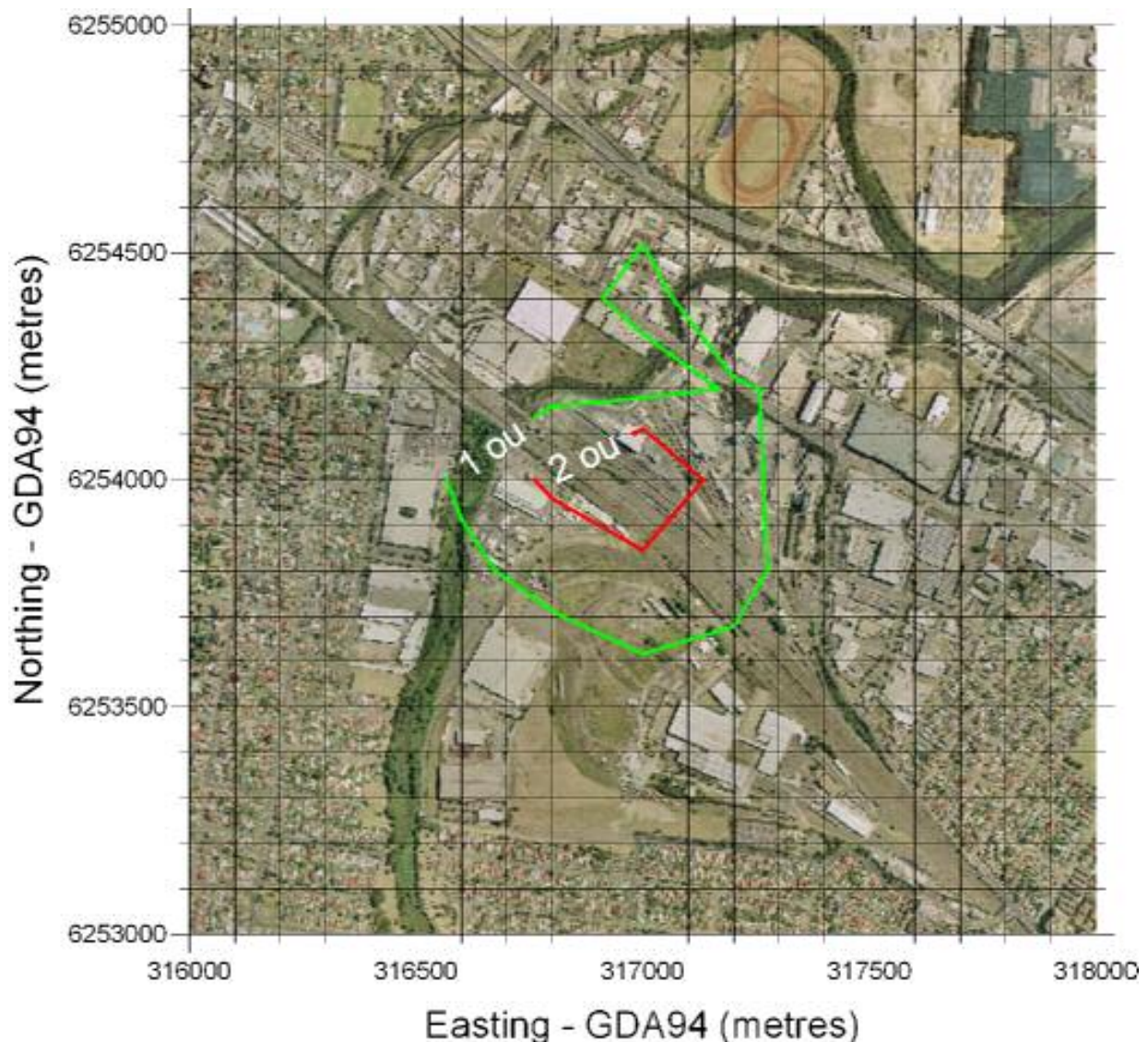
Figure 3.2: Scenario 2 - Projected ground level odour concentration contours for the Veolia ES Waste Transfer Terminal Building at Clyde from a 21m high stack and a 17m high building.
