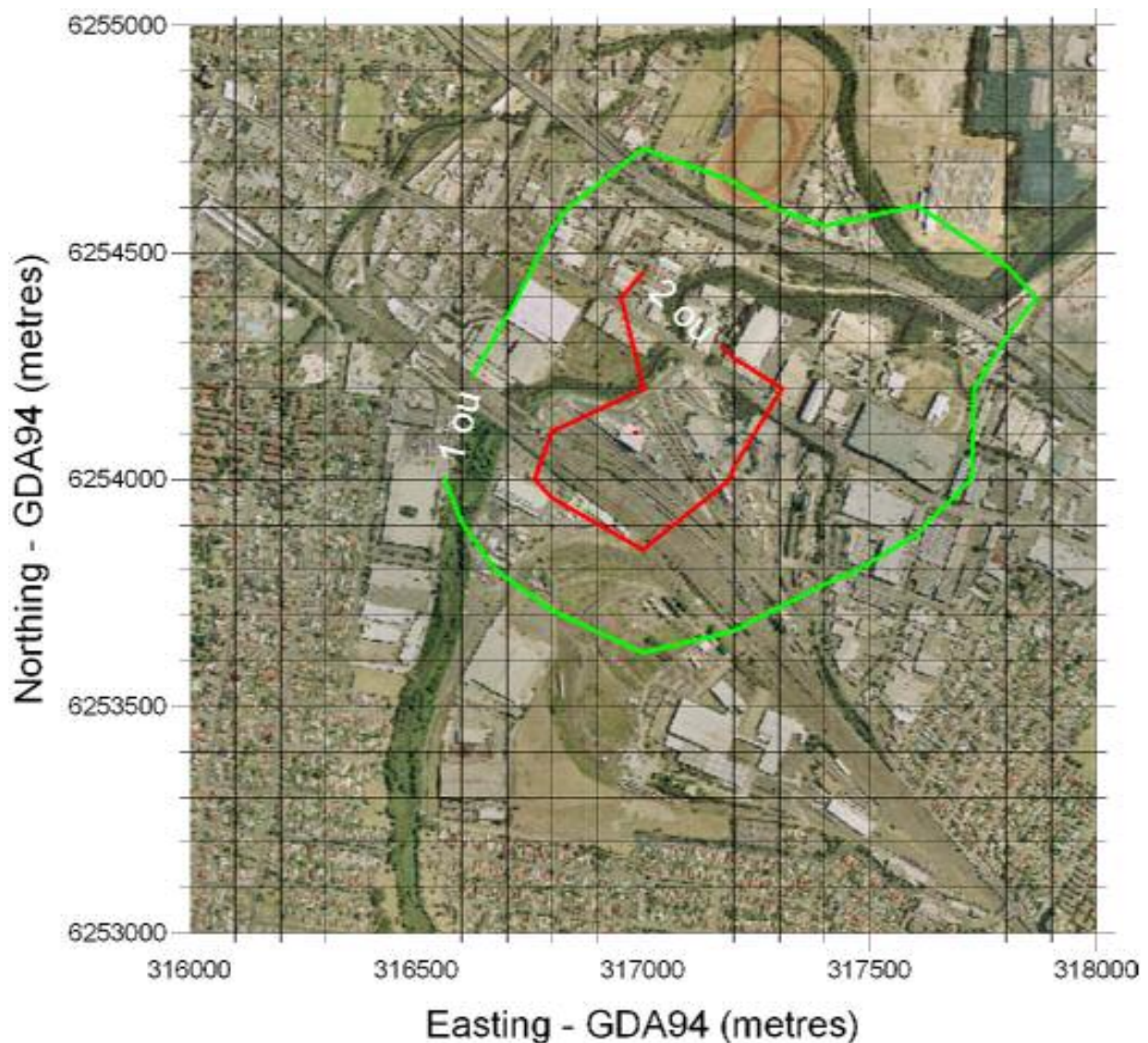
Figure 3.4: Scenario 4 - Projected ground level odour concentration contours for the Veolia ES Waste Transfer Terminal Building at Clyde from a 21m high stack and a 17m high building.
