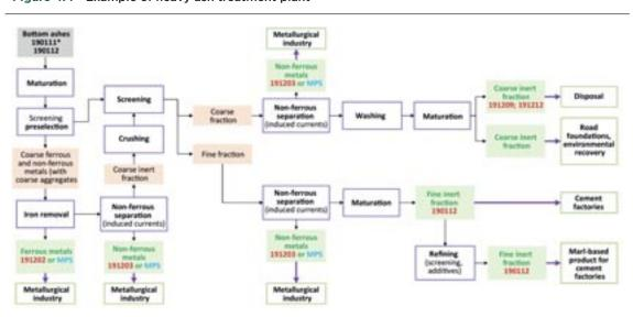
Figure 4.4 - Example of heavy ash treatment plant
