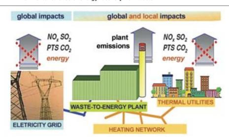
Figure 4.1 - Environmental balance of energy recovery from waste
