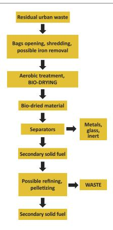
Figure 5.2 - Diagram of an MBT with biostabilisation process
