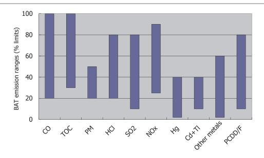
Figure 3.2 - Comparison of emission measurements during three-year period 2016-2018 in Italian plants and ranges associated with BAT levels for conventional (a) and trace toxic contaminants (b).
