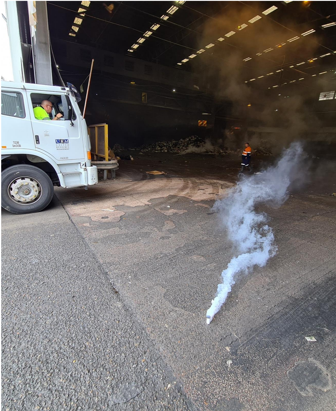
Photo 2.4 – A view of the truck entrance plastic strips during smoke testing on 25 November 2021
