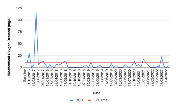
Figure 2.13 - BOD trends in stormwater discharge
