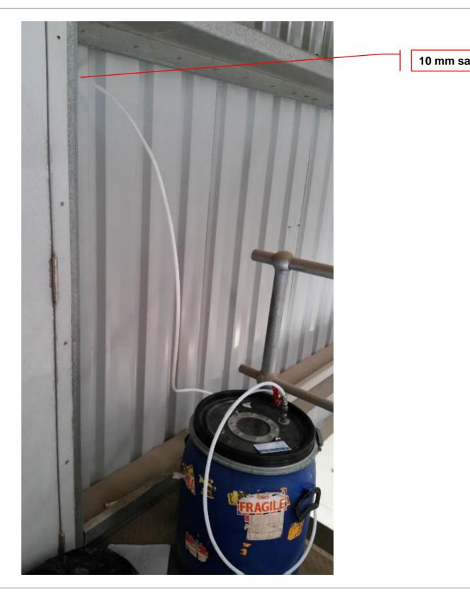
**Photo 1** – An example of the roof discharge stack odour sampling point at the BTT Facility
