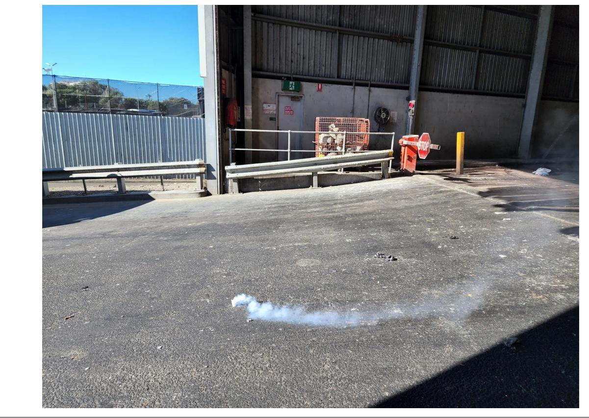
Photo 2 – Smoke testing at the truck entry point of the BTT Facility building enclosure on 1 June 2022
