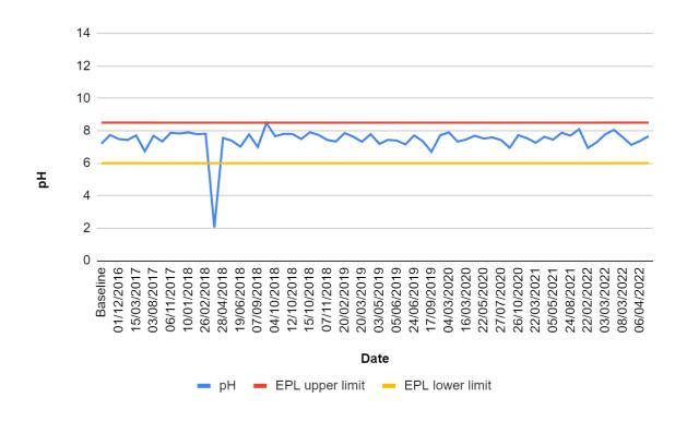
Figure 2.10 - pH trends in stormwater discharge
