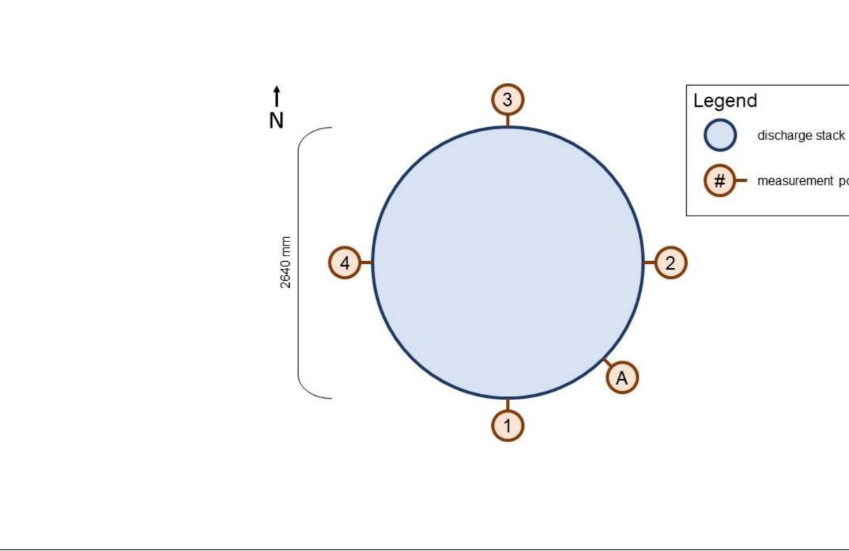
Figure 2 – Diagram displaying a cross-sectional view of the roof discharge stack and location of measurement points
