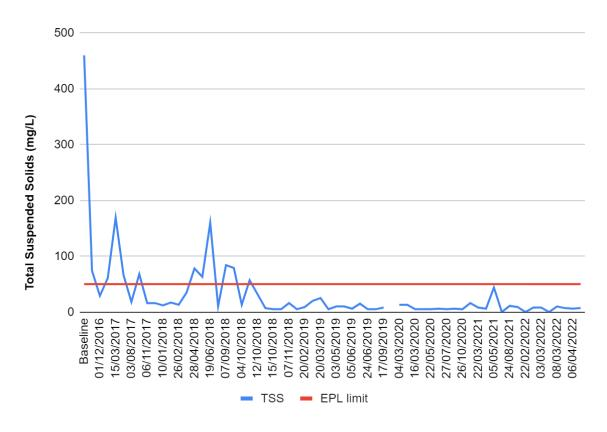
Figure 2.11 - TSS trends in stormwater discharge
