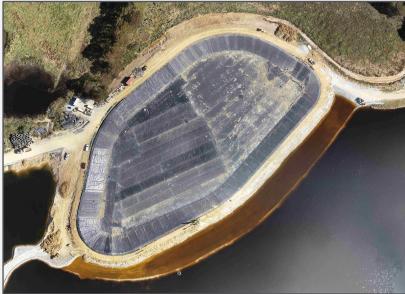
Coffer #2 2023 and start spray discharge for better evaporation
