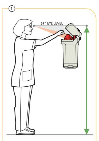
Identify the location and height for the container placement. Place the wall mount flush against the wall and level it from side to side and back to front. An ideal standing installation height for a fixed sharps disposal container is 1.35m. This height will comfortably accomodate 95% of all adult female workers.
