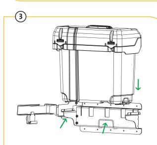
Place the container in the bracket coming down from the top and hooking the container in the back catch bar and side support brackets.
