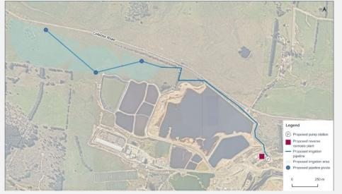
Proposed modification to put in an additional water treatment step = ~50% ultra pure water for beneficial water e.g. for use in water carts, irrigation to the onsite farm, washdown processes, operational processes onsite and the remaining goes to leachate dams.
