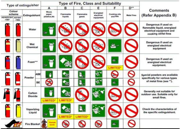
Limited indicates that the extinguishant is not the agent of choice for the class of fire, but that it will have a limited extinguishing capability.
