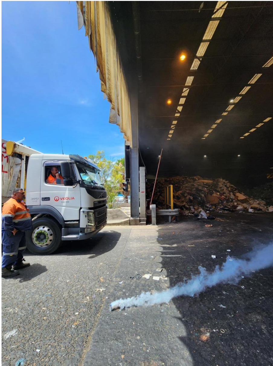
Photo 2.4 – A view of the truck entrance plastic strips during smoke testing on 21 December 2022
