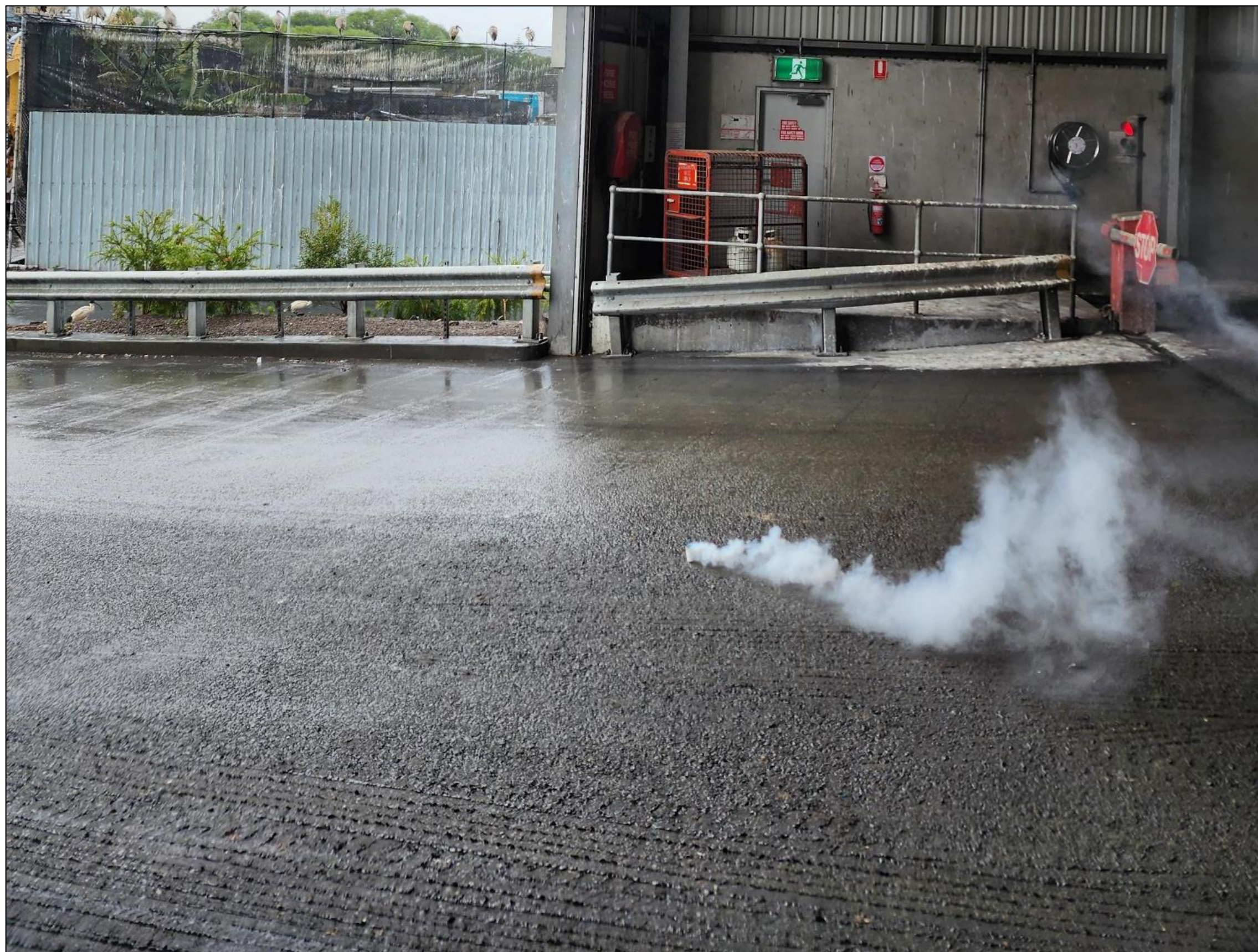
Photo 2 – Smoke testing at the truck entry point of the BTT Facility building enclosure on 4 July 2023
