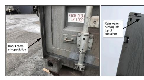
Rainwater can accumulate on the roof of the container and run down the sides during transit, especially when encountering hills or cornering. A review of historical rainfall data for both Sydney and Goulburn confirmed rainfall on 17 January 2024, and the preceding days, which coincides with the timeframe when the container was transported to Woodlawn.
