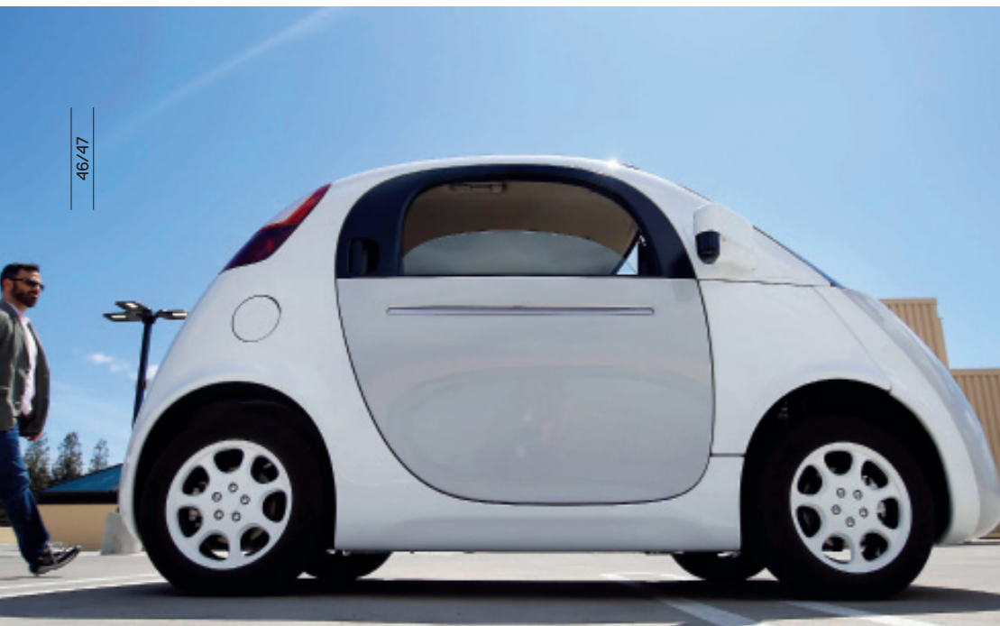
The new Google Car boasts a host of sensors and artificial intelligence, including a laser remote detection system, radars, camera, receiver, etc. The prototypes do not have a steering wheel, accelerator or brake pedals. However, these devices will be fitted to self-driving vehicles traveling on California's public roads this summer!
