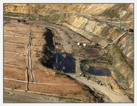
**After**: Filled area installed drainage and gas capture infrastructure. Waste face will be caly lined and gas infrastructure installed.
