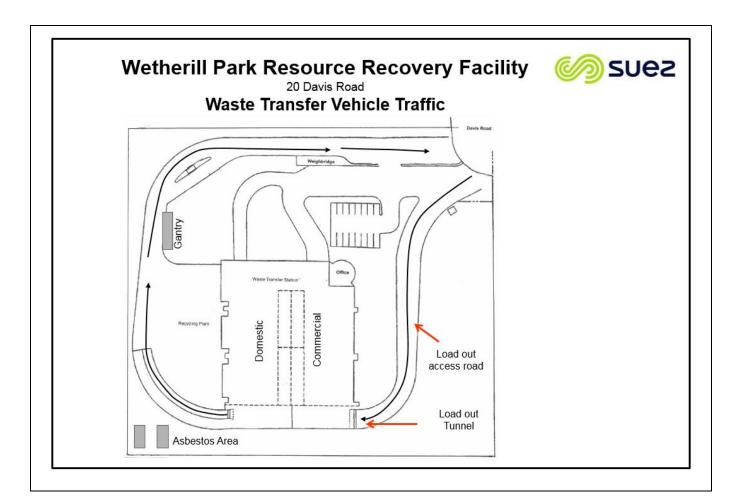
Diagram 10 - Waste Transfer Vehicle Traffic
