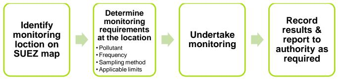
Figure 3 Summary of the monitoring process at Wetherill Park Resource Recovery Facility.
