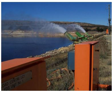
Figure 1: Evaporator units in action
