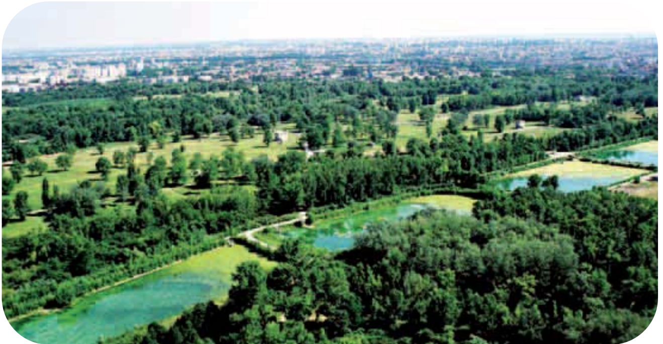
The Crépieux-Charmy abstraction zone and the infiltration basins for aquifer replenishment located in the centre of Lyon, France
