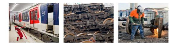
RATP has chosen Veolia to dismantle and recycle 317 RER A line passenger cars. Dismantling these rail cars is possible thanks to the expertise and complex technical knowledge Veolia is putting into place for RATP. It will enable 97% of the materials in these passenger cars—each measuring 25 meters long and weighing more than 30 metric tons—to be recycled and recovered. This is a first in France for an operation of this size.
