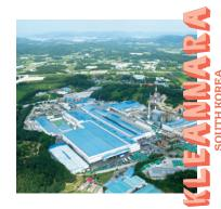
The Korean paper manufacturer Kleannara has entrusted Veolia with the management of water treatment (59,000 m³ of water per day) and wastewater (28,000 m³ per day) facilities on its Cheongju site. The Group also operates two boilers, producing 42.5 metric tons of steam per hour; the solid fuel used comes from the plant's production process. This circular economy loop significantly reduces the plant's environmental footprint.
